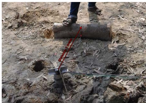
Figure 2.4 Calculation of Shear Wave Velocity by Down hole Seismic, where R=Distance between source to geophone
