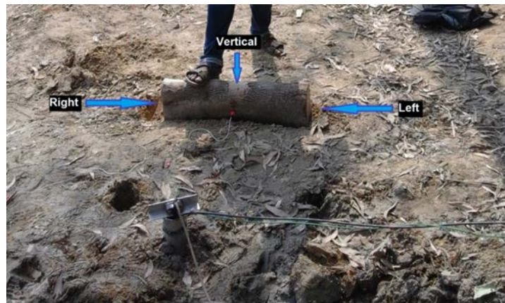
Figure 2.10 Hit the wooden plank in 3 directions which are on the left, right and vertical directions.
