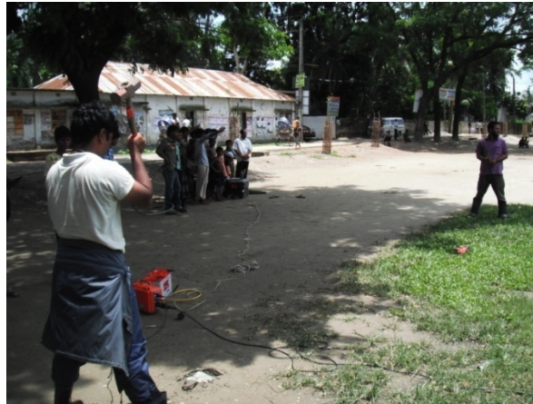
Figure 2.18 MASW Field Data Acquisition
