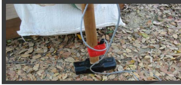
Figure 2.6 To attach the trigger to a hammer.
